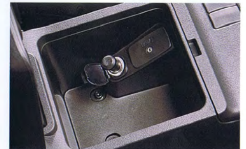
63 Cigarette lighter kit H6710FG000 W Changes the accessory socket to a cigarette lighter.
